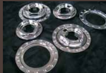
Laser sinter parts chrome optics, sealed with clear coat
