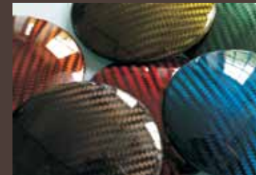
Carbon samples colour glazed, sealed with clear coat
