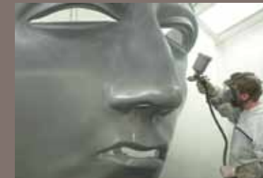
Varus mask, museum Kalkriese GFK, aluminium coating, polished
