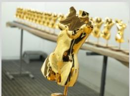
With given construction data and design we prepare the substrate and specially treat the objects with regard to the perfect finish. The final finishing touch is delivered by precision grinding, high-gloss polishing or nano-sealing
