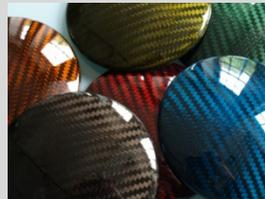
Upgrading Carbon parts with unique effects. The carbon fibres are being enhanced by user-defined colours and grade of glossiness. A special primer and clear coat ensure durability und light-resistance.
